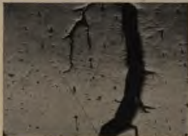
No. 46. SLAG CRACK IN SOLID SECTION OF TIRE.
